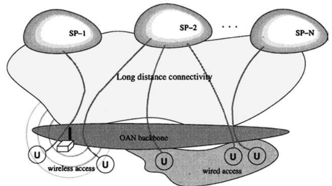
Figure 1. Basic logical structure of an OAN based telecommunication service, the OAN supports any SP and any authorized user through wired or wireless access.
